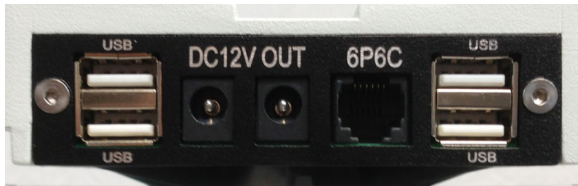
Figure 5. Cable management panel
