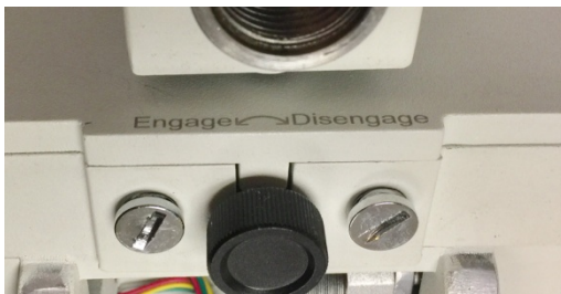
Figure 4. CEM60 R.A. (left) and DEC (right) gear switches
