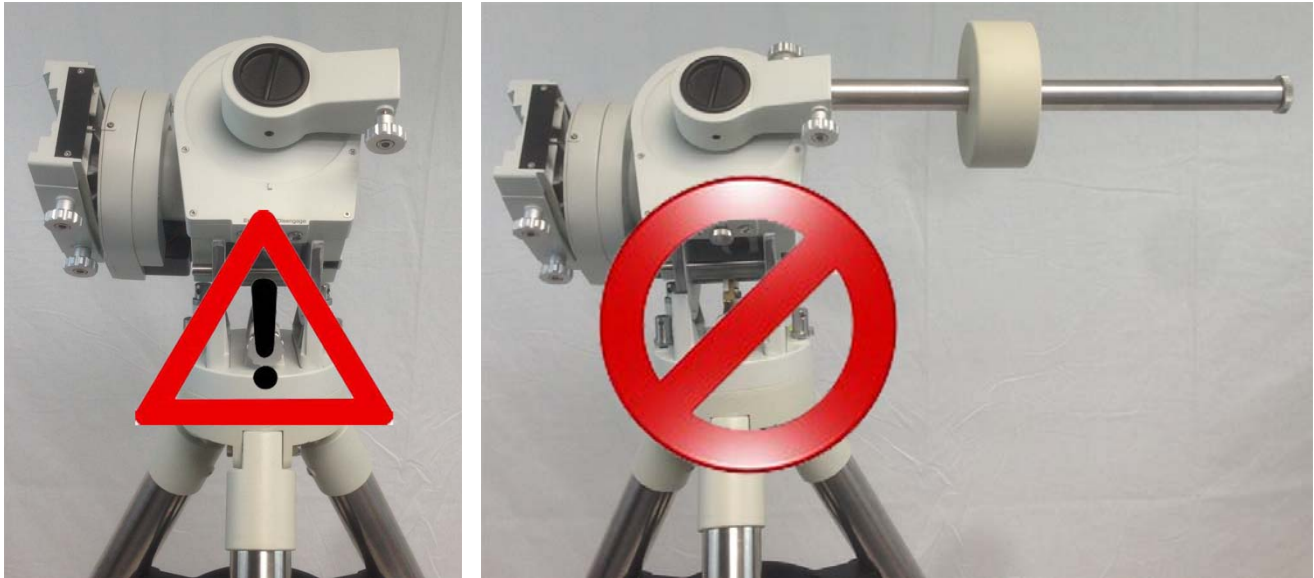
Figure 12. Do not operate the mount with an unbalanced load, for instance with a counterweight installed without an OTA, as shown above, or vice versa
