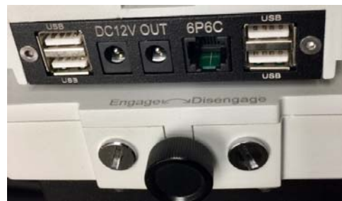
Figure 4. CEM60 R.A. (left) and DEC (right) gear switches
