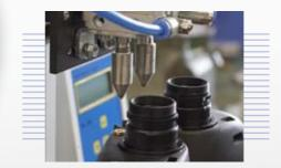
Fogging up or the formation of condensation inside the binoculars is totally prevented by this high-tech proprietary solution. Even temperature variations between -40 °C to +80 °C do not affect the functionality of STEINER nitrogen-filled binoculars. By 2-way-valvetechnology, the maintenance of the binoculars is possible at any time even after many years.
