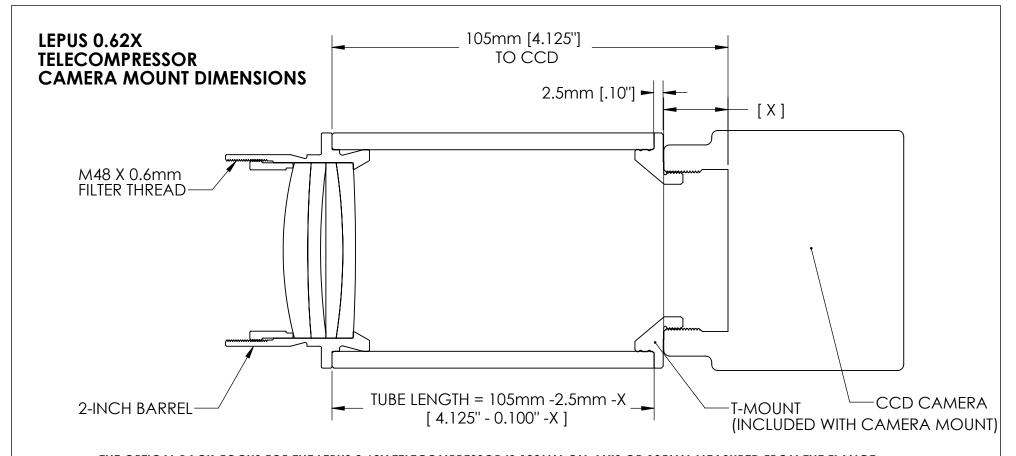
THE OPTICAL BACK-FOCUS FOR THE LEPUS 0.62X TELECOMPRESSOR IS 100MM ON-AXIS OR 105MM MEASURED FROM THE FLANGE.
