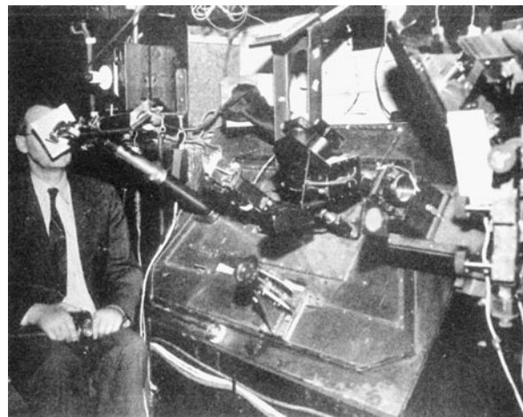
Figure 1.5. Auxiliary equipment at the coude focus of the Mt Wilson 100-inch telescope. Ira Bowen is guiding a star on the slit, while shielding his eyes with the mask from the glare of the iron comparison arc.
