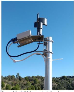
Image of the AAG & Anomometer in the pole mounting bracket.
