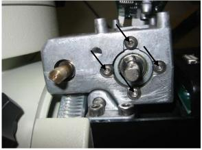
7. Remove the periodic error (PE) reference encoder from the RA house.
