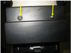
3. Unscrew four screws on the RA motor drive board.
