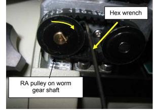
4a. In order to turn the pulleys, you need to partially disengage the worm gear. Make sure the power is turned off. While pushing down on the edge of the RA gear box, turn the RA pulley to access the set screws with a hex wrench.
