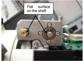
21. Remove the set screws from old RA shaft pulley and install it onto the new one. Adjust the
