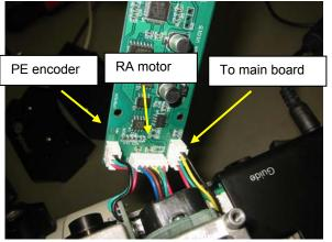
6. Loosen the four screws that secure the motor and remove the motor from the RA worm gear house from the other end.
