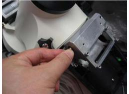
19. Install the new PE encoder wheel and board. Then reinstall the RA motor. Tighten the four screws evenly. Install the RA board and connect the cables.
