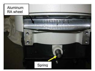
9. Remove the hinges (different on each side) from hinge shaft. Be careful not to lose the two copper washes that go with the hinges. Remove the PE encoder wheel from the RA worm shaft by releasing a set screw on the wheel.
