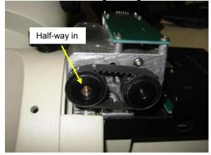
23. Turn the mount in RA direction in full speed to see if the mount is running smooth and well. If a multimeter is used to measure the slew current, it should be less that 600mA while slewing at MAX speed. The smaller the reading, the better worm and wheel mesh. Secure the RA board and replace the cover.
