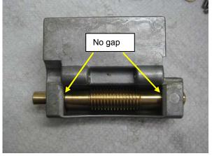
16. After the end cap is fully tightened, release 1/8 to 1/4 turns of the end cap. Turning the worm gear to make sure it turns smoothly and there is no plays introduced while pull the worm end. A little stiffness is OK. Secure the set screw. Apply some grease as needed while assembling.
