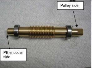
15. Install the end cap. When tightening the end cap, make sure there is no gap between the bearing race and shaft inner edge wall, as indicated in the photo.
