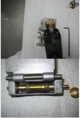
12. Pull the RA worm and 2 bearings out of the house. Lightly tap the end if needed.
