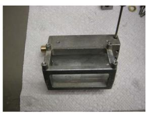
17. Insert the hinge shaft into the RA house. Place the copper washers and hinges back onto the shaft.
