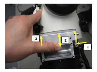
Turn the RA worm gear shaft to rotate the mount along RA axis. It should easily move in both directions. If not, the cage position needs to be adjusted.
