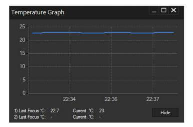
You can easily check when was the last focus temperature so you can know exactly if it is time to refocus.
