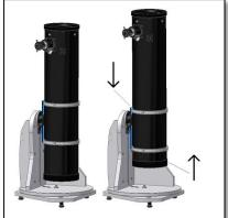
Figure B. Move the dovetail down and the tube up!
