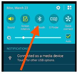
Figure 6. Enable the Bluetooth® function.
