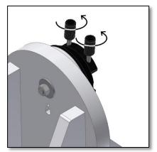
Figure A. Release the two dovetail knobs (part 1)
