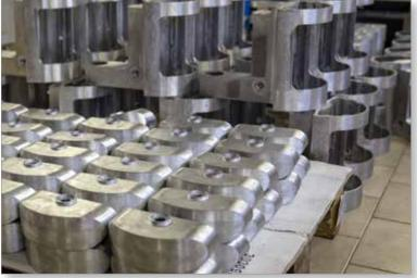
Microscope stands exiting from the internal varnishing facility.
