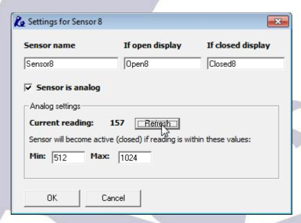
... as the image shows. Clicking "refresh" will update the current reading. The goal is determining the range of values where we can consider the object is in its place; in our example, the mount is parked, so we could:
