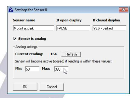
... the main Dragonfly window will update its display accordingly to the current position of the mount. As seen, we've also filled the rest of the fields (sensor name etc), and used sensor number 8 as it is more convenient due to the ground plugs placement. There is a separate instruction sheet for wiring this kind of sensors, just check our web site.
