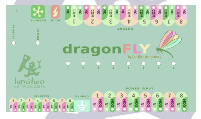
... you'll note we've used this naming convention for labeling the input and output connectors.
