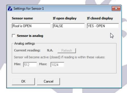
for the roof (roll off roof) we suggest using two switches, one for signaling "open" and other to signal "closed", this way we will notice should the roof stop mid-travel.
