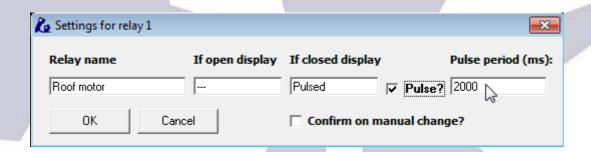
You can name the relay and what should appear when it's closed and open. You can also define it to be a "pulsed" relay, as appropriate in the roof motor configuration. The pulse period, you surely guessed it, is the approximate duration of the pulse in millisecods.
