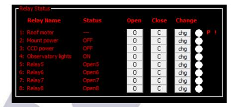
Notice both the "P" and the "!" at the right side, roof relay; the "P" means it is pulsed, the "!" means you'll be asked for confirmation before any action takes place.
