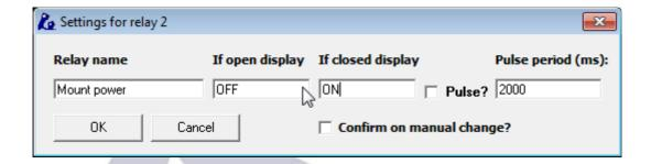
... please continue to do the same for the CCD power and observatory lights – don't forget the lights will be forced off if the relay is closed!
