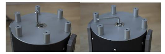
Tighten firmly with enclosed Allan Key - do not over-tighten.
