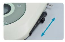
The OCC illuminator can be controlled using a slide lever. Thanks to scales on the slide lever, the user can save and reproduce desired illumination levels. In addition, an OCC plate can be inserted into the illumination unit from the front and rear sides, so images with different shadow direction can be observed.
