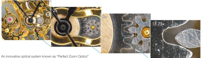
An innovative optical system known as "Perfect Zoom Optics" offers the world's first zoom ratio of 25:1 (zoom range: 0.63x - 15.75x). The SMZ25 can seamlessly capture the entire dish while simultaneously delivering microscopic details.
