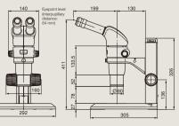
SMZ1270 set SMZ1270 + P-B Binocular Tube + Plan Apo 1x/WF + P-PS32 Plain Stand
