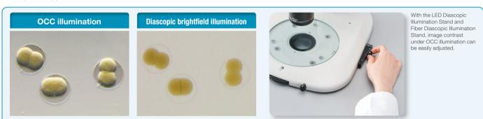
OCC illumination boosts the contrast of transparent sample structures. Hemicentrotus pulcherrimus in two-cell stage
