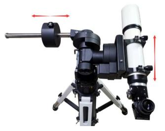
CAUTION: The balancing process MUST be done with Gear Switch at the total disengaged position! Otherwise it might damage the worm system.
