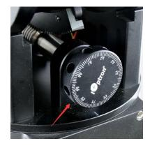
4. <u>Install counterweight (CW) shaft</u>: The CW shaft system is a two part configuration. It comes with preinstalled top part of the shaft. Just simply thread the CW shaft onto it.
