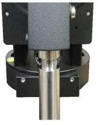
5. Install counterweight(s): Before putting on CW, make sure the mount is at its zero position, i.e., CW shaft points to the ground. Disengage the R.A. Gear Switch to set the R.A. axis free before loading the CW. Remove the CW Safety Cap at the end of CW Shaft. Glide the CW over the shaft with the larger hole opening facing down. Place the Safety Cap back onto the shaft. Move the CW to the bottom of the shaft and tighten the CW locking Screw.
