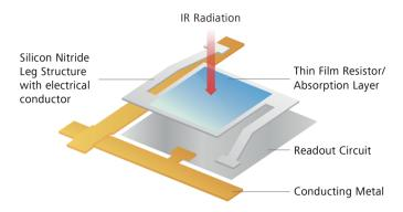
Schematic illustration of a microbolometer.
