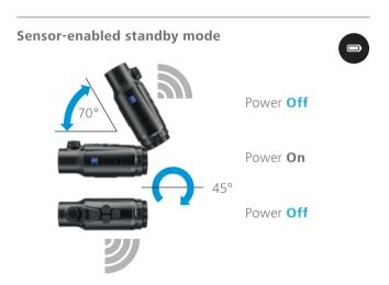
The angle sensor automatically detects the exact position of the ZEISS DTC 3 and activates standby mode at a lateral angle of 45° and at a downward or upward angle of 70°. When the hunter brings the weapon back to the firing position, the device automatically exits standby mode.
