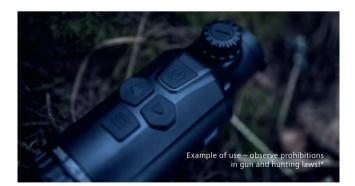
With a field of view of 18.4 meters at 100 meters, the ZEISS DTC 3/25 provides the best overview for night hunting in forested areas.
