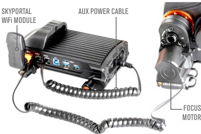
FIG. 3: AUX POWER CABLE POWERING ADDITIONAL ACCESSORIES
