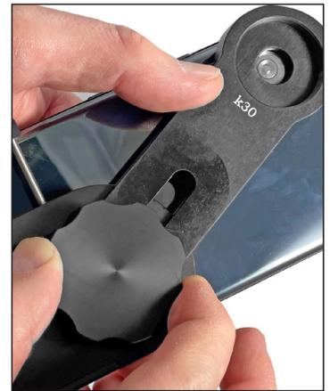
4. Once alignment has been achieved, secure the Opticsrail (I) by turning the locking wheel (A) clockwise until it is secured in place.
