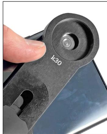
3. Loosen the locking wheel (A) and then rotate the Opticsrail (I) so that the hole sits central over the lens of your smartphone camera. If your smartphone has multiple lenses - simply align the hole with the lens you want to use.
