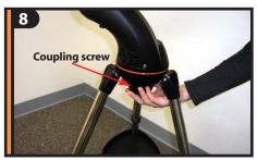
Thread the coupling screw into the hole at the bottom of the fork arm base. Tighten screw to secure the entire fork arm.
