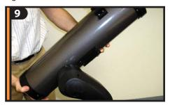
Slide the optical tube dovetail into the fork arm as shown above.
