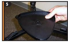
Place accessory tray on top of center leg brace by lining up the grooves on the tray to the post on the brace.
