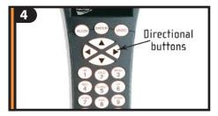
Use the hand control direction arrow buttons to point telescope at a distant land object, like a telephone pole or at night you can use the moon. Center and focus the object in the 25mm eyepiece of the telescope.
