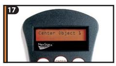
The hand control will prompt you to center the bright alignment star in the center of the eyepiece. Once centered, press ALIGN. This will accept the star as your first alignment position.
