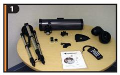
Your NexStar 130SLT includes: optical tube; fork arm; pre-assembled tripod; computerized hand control; hand control holder; two eyepieces; finderscope; accessory tray; documentation including an owner's manual, The Sky® CD and NSOL Telescope Control Software.
