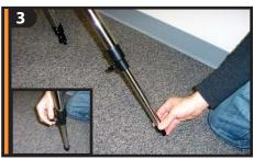
Extend tripod legs 6 to 8 inches by loosening the tripod leg locking knob and pulling the leg to desired length and re-tightening knob.
