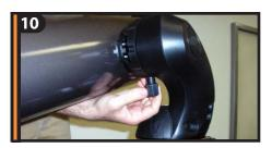
Secure optical tube to fork arm by tightening the screw located on the inside of the fork arm assembly.
