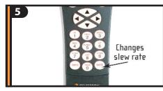
In order to accurately center an object in the eyepiece it may be necessary to change the slew speed of the motors. To change the slew speed, press the RATE button then select a number from 1 (slowest) to 9 (fastest).
