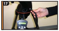
Plug Computerized Hand Control into the "Hand Control" port on the fork arm.
