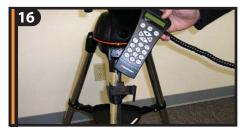
Slide Computerized Hand Control into the hand control holder as shown above.
