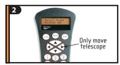
You will notice that there are directional arrows in the center of the hand control. These **only** move the telescope. **They cannot be used to scroll through menu features.**
