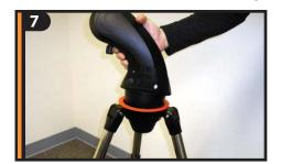
Hold the telescope fork arm and place the bottom of the base inside the tripod mounting platform as shown.
