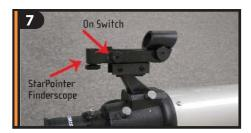
Once you have aligned your finderscope, make sure to turn off the LED light to conserve the battery. Now you are ready to align the telescope. This will have to be done at night.
