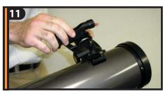
To attach the finderscope, loosen the silver screw and slide finderscope into mounting platform.
